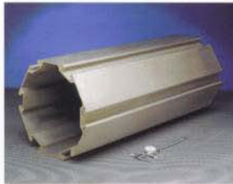
Thirty inch long tooling for a fiberglass reinforced telephone pole
